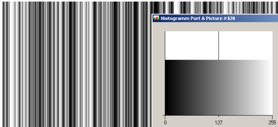
Figure 4.17: LFSR test pattern received at the frame grabber and typical histogram for error-free data transmission
