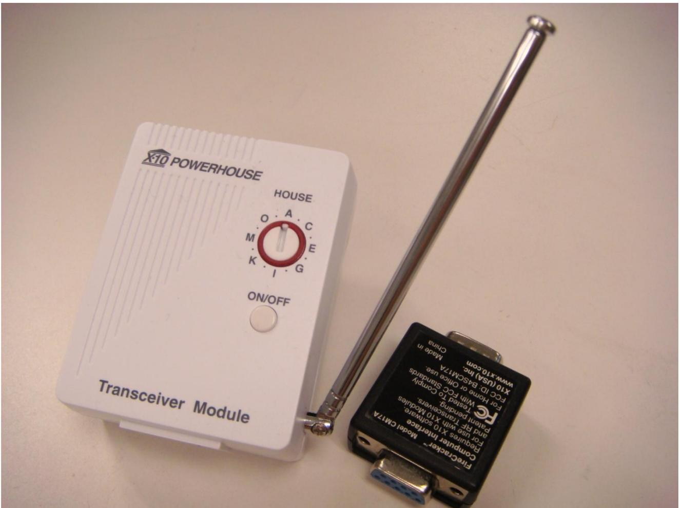
**Step 1:** Locate the X-10 wireless transceiver. Note the house letter assigned to the device.
