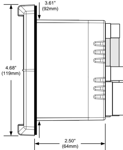
**Figure 13. Case Dimensions – Side View**
