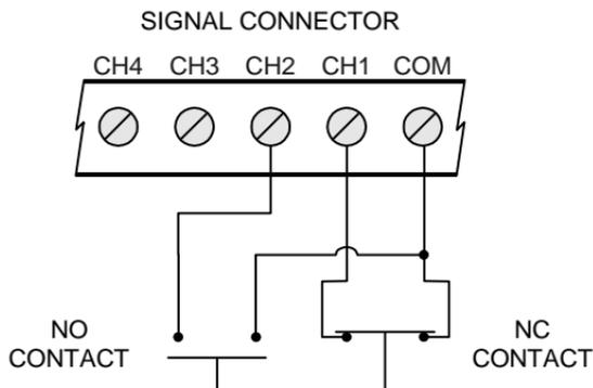
Figure 4. NO/NC Contact Inputs
