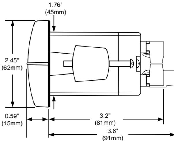
**Figure 14. Case Dimensions – Top View**
