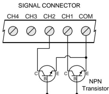
**Figure 5. Open Collector NPN Transistor Inputs**
