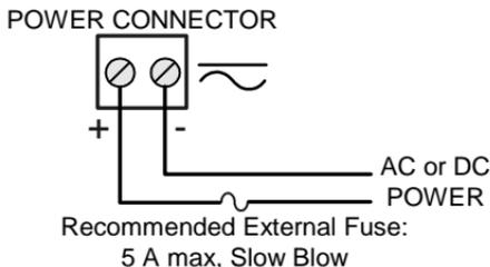
**Figure 3. Power Connections**
