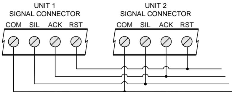
Figure 11. Shared Pushbutton Connections
