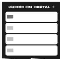
5. Press **RESET** to change LED 1 from off to on, setting channel 1 for a NC input.
