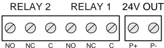
**Figure 6. Relay & 24 V Output Connections**
