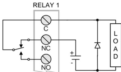
Use a diode with a reverse breakdown voltage two to three times the circuit voltage and forward current at least as large as the load current.
