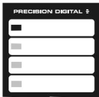
4. LED 1 will be off indicating normal operation of relay 1. LEDs 2 through 4 will be dim.
