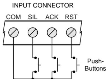
**Figure 9. External Pushbutton Connections**
