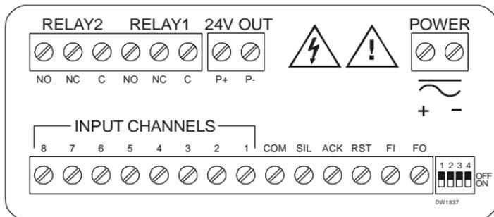
**Figure 2. Connector Labeling for PD158-6R2-1**
