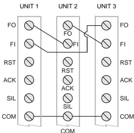
**Figure 10. System with Multiple Units Share First-Out**
