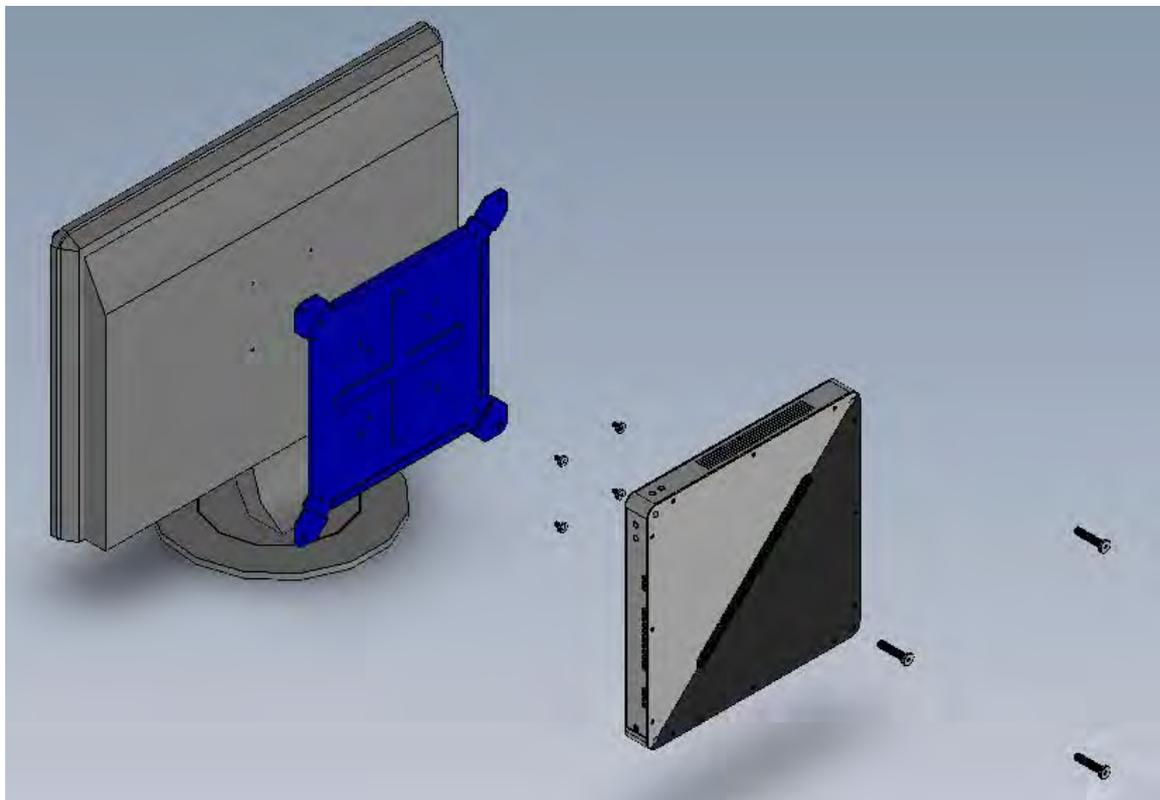
You can install SI-58 on plastic (LCD monitor), wood, drywall surface over studs, or
