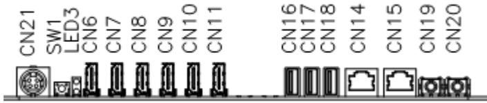
**CN6, CN7, CN8, CN9, CN10, CN11: ATI E6760 HDMI Connectors**
