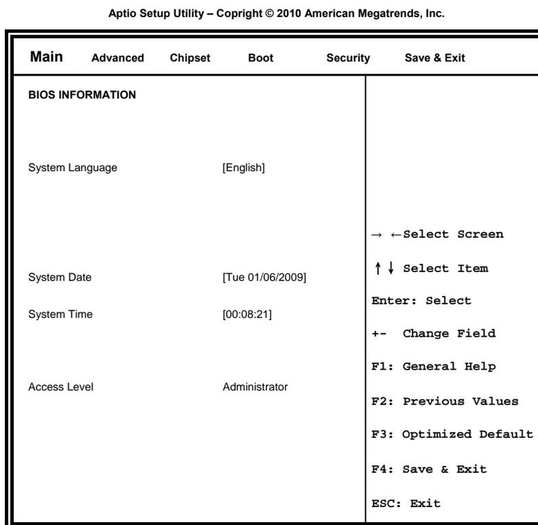
**Note:** *If the system cannot boot after making and saving system changes with Setup, the AMI BIOS supports an override to the CMOS settings that resets your system to its default.*
