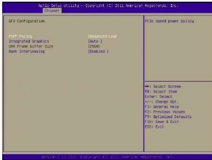
Figure 3.13 GFX Configuration Screen
