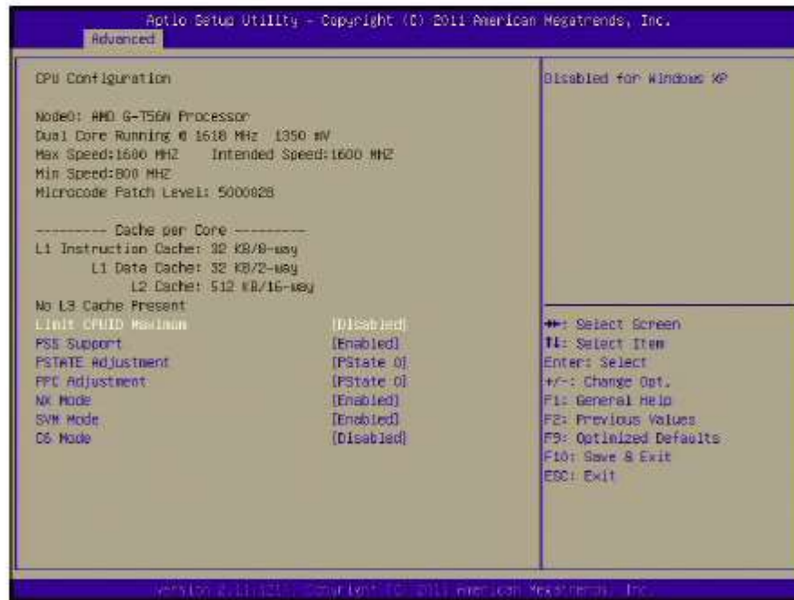
Figure 3.5 CPU Configuration Settings Screen
