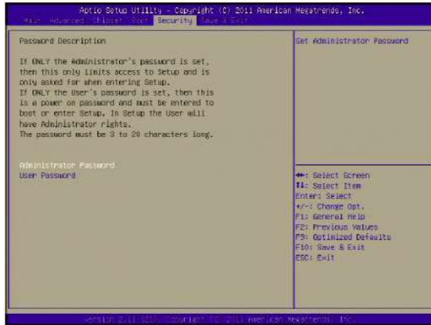
Figure 3.18 Security Setup Screen
