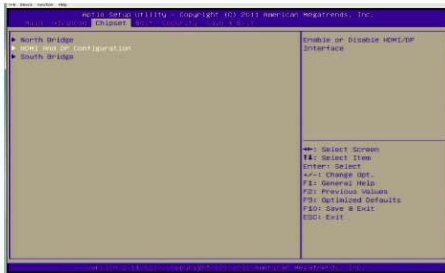
Figure 3.11 Advanced Chipset Features Screen
