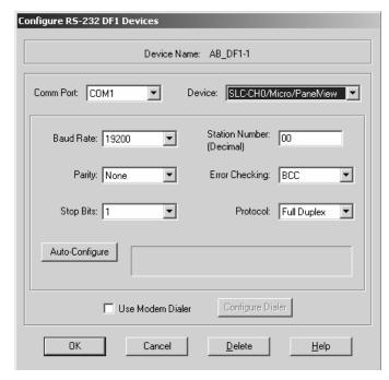
To use the auto configure you must first select the device as SLC-CH0/Micro/PanelView.
