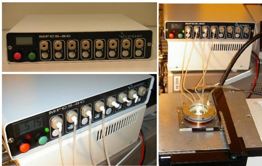
**Figure 1: Top Left: 8-channels MFCS; Bottom left: 8 channels MFCS with pneumatic connections. Right: Typical experimental microfluidic work station consisting in the MFCS, a chip holder, and an epi-fluorescence microscope (computer not shown).**
