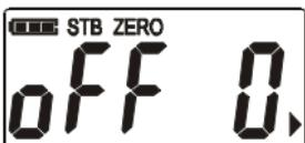
Press **HOLD/UNIT** to change Auto-Off option. Auto-Off can be set to 0min (never), 5min, 15min, 30min, 60min.
