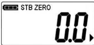
Zero the scale. ZERO is shown. Weight reading turns "0.0" or "0.00". The relative indicator on the display turns on.
