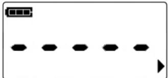
The screen shows detection message while scale detects its load and auto-zero itself.
