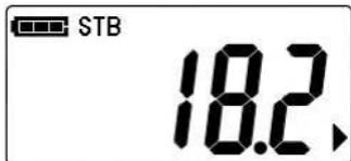
HOLD is hidden. Weight reading is unlocked.
