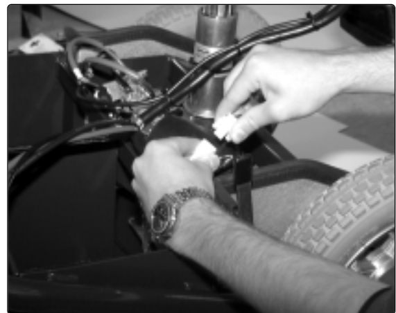
The magnetic brake's electrical connection
