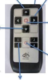
**Speed Settings:** Preset buttons for specific speeds. 1 is the slowest, 4 is the highest. See programing to change speed settings.
