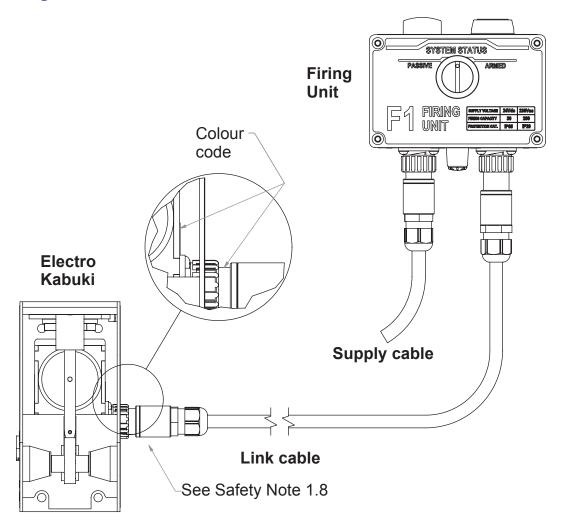
Care should be exercised in the support and routing of the link cable between the Firing Unit and the Electro Kabuki in order to minimise strain on the connections and prevent the cable forming a tripping or choking hazard.
