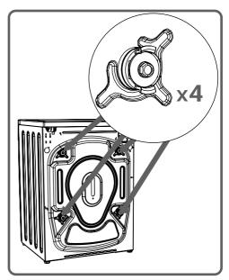
For this reason, transportation safety screws shall be loosened by being rotated in counter-clockwise direction using an appropriate wrench.
