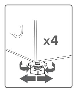
• Never put cardboard, wood or suchlike materials under your machine if you are intending to level the appliance on the floor surface.
