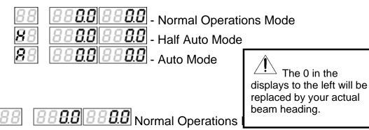
In Normal Operations Mode, the  $\leq$ ,  $\land$ ,  $\lor$ ,  $\triangleright$  buttons cause rotation as long as the buttons are pressed. Pressing S while in normal operations mode will take you to setup mode.
