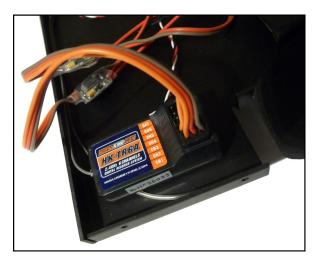
18. Time for a test! Make sure the power plug is inserted in the bottom of the robot (so the robot is off). Set the robot on something so that the wheels are off the ground.
