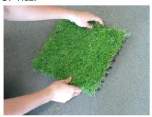
2. FOLLOWING THE SAME FIBRE DIRECTION, PLACE NEXT TILE TO THE RIGHT OF THE FIRST TILE WITH MALE INTERLOCKING CLIPS ON RIGHT SIDE INSERTING INTO FEMALE INTERLOCKING CLIP. ONCE INTERLOCKING CLIPS ARE INLINE PRESS DOWN FIRMLY TO LOCK TILE.
