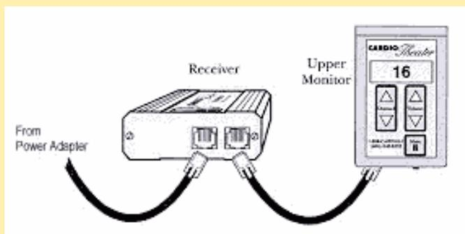
**Receiver powered by machine with Upper Monitor Box:** For cardiovascular equipment that IS Cardio Theater ready, power will be supplied via a connector on the cardiovascular equipment. An Upper Monitor Box is then attached to the receiver.
