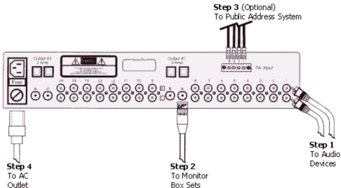
**NOTE: MAKE ALL CONNECTIONS TO MAIN AMPLIFIER, UPPER MONITORS & AUDIO DEVICES WITH POWER OFF.**
