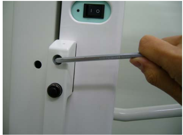
Fix by a cap screw M6×40.
