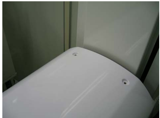
Fix with two truss screws M3×8.
