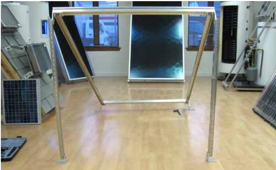
Step 28: At this point the entire assembly may be flipped over and stood up as shown.
