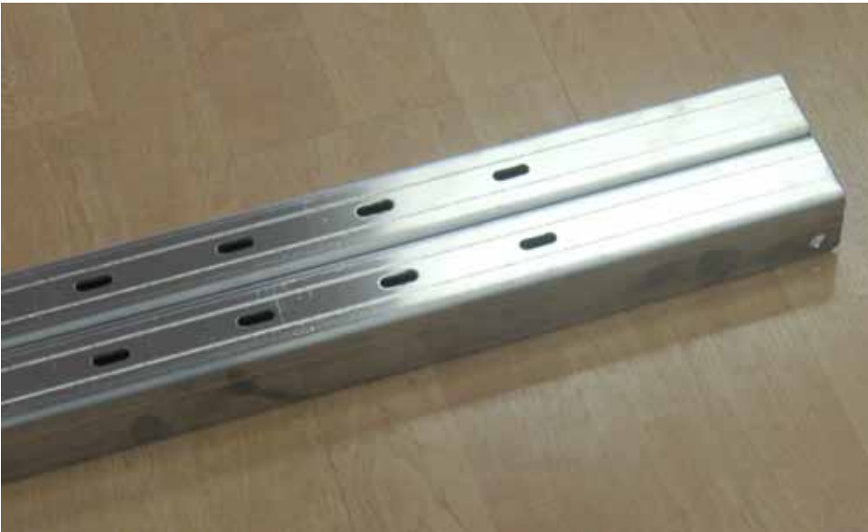
Step 13: When performing assembly steps involving the base support, make sure to use the same end of said supports for analogous parts of each half of the assembly, as they appear to be symmetrical but are not. To check, line them up as shown. This is the correct orientation.
