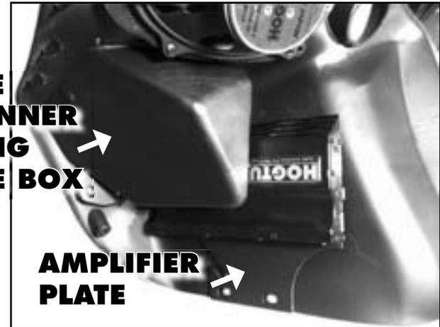
Diagram 1.1 (Amp mounts to brake side of inner fairing "behind" glove box)
