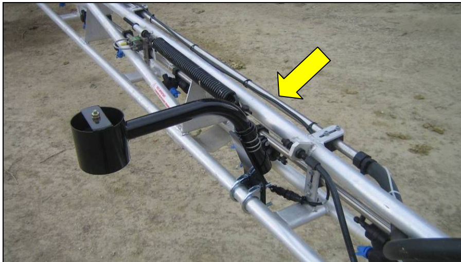
Figure 9: Sensor Bracket Mounted to Boom, Near the Break-Away Spring.
