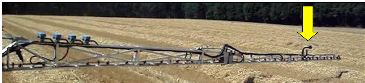
Figure 10: Location of Sensor on 28m TR4 Boom
