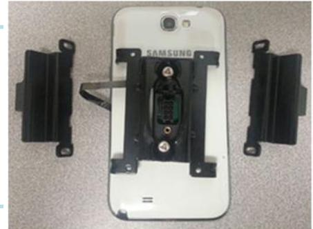
2. Attach side security brackets and secure with screws
