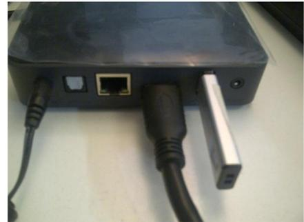
4. Ensure the WDTV is turned off before removing the old key and replacing it with the new key.
