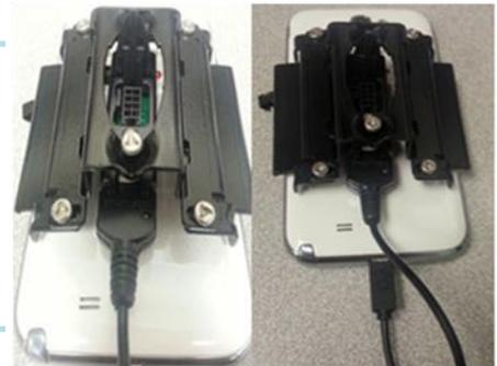
5. Plug Retractor into Disc Sensor
