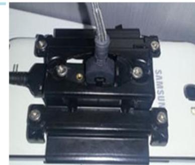
3. Using the Tri-wing Security Key unscrew security screws from brackets
