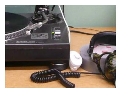
5. Setup the haptic floor under the desk. The haptic floor includes both the vibrating tiles and the amplifier(which also acts as a low-pass filter). We amplify the bass so that you feel the beat and soften the treble so that it is not audible to the audience.
