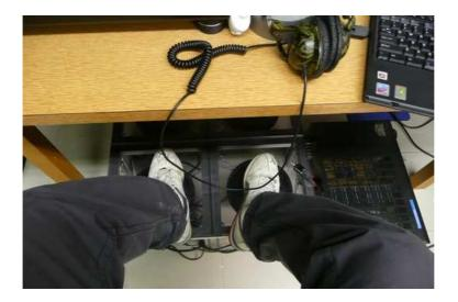
6. Connect the stereo splitter into the audio-out of the computer. One channel is for the haptic floor, one channel is for the channel splitter.
