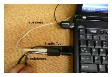
7. Plug the computer speakers into the L-channel of the splitter and headphones into the R-channel.
