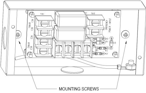
Wire the Low Voltage Transfer Module as shown (See page 3 for installation with a dual lamp lighting fixture). A grounding lead is supplied inside the housing. Replace cover. Emergency unit equipment used in the installation must be 12VDC output and of equal or greater wattage capacity than the lighting fixture requires (Max. 75 watts per channel). Test for proper function by shutting off main AC feed and checking for continued lamp lighting.
