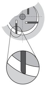
In case the vanes (35) are undamaged, the height A of all vanes is more than 23 mm and regular inspections in short intervals are ensured:
