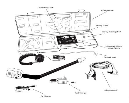
**Theory of Locating** - Cable Locators consist of a transmitter and a receiver. In the case of the Pro800, the transmitter is the long black box and the wand is yellow and black. In operation, a transmitter places a specific frequency signal onto the metallic conductor you are trying to trace. This placing of an AC signal onto a cable produces an electrical current and an electromagnetic field around that cable. If the wand is close enough, this signal is received and amplified by the wand.
