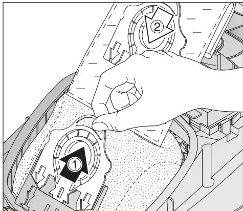
An empty-operation-barrier blocks the dust compartment lid from closing if no dustbag is inserted or if it is not inserted all the way. Do not force it closed.
