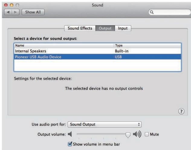
If the [Pioneer USB Audio Device] does not appear, confirm that the **DIGITAL IN USB** port has been selected as input source. Then try reconnecting the cable or turning the power off and then on again; when this is done, the [Pioneer USB Audio Device] should be recognized.
