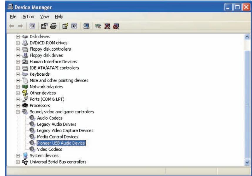
If the [Pioneer USB Audio Device] does not appear, confirm that the **DIGITAL IN USB** port has been selected as input source. Then try reconnecting the cable or turning the power off and then on again; when this is done, the [Pioneer USB Audio Device] should be recognized.
