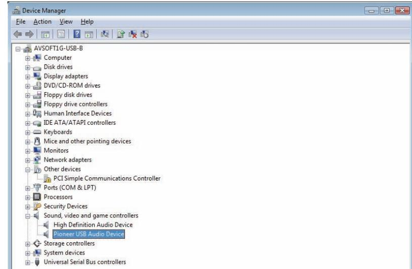
If the [Pioneer USB Audio Device] does not appear, confirm that the **DIGITAL IN USB** port has been selected as input source. Then try reconnecting the cable or turning the power off and then on again; when this is done, the [Pioneer USB Audio Device] should be recognized.
