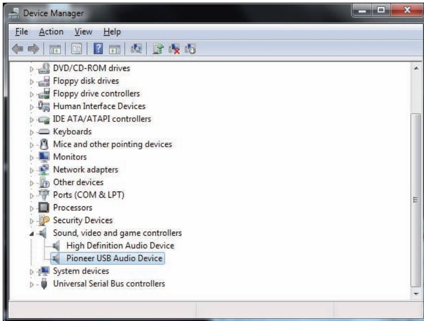
If the [Pioneer USB Audio Device] does not appear, confirm that the **DIGITAL IN USB** port has been selected as input source. Then try reconnecting the cable or turning the power off and then on again; when this is done, the [Pioneer USB Audio Device] should be recognized.
