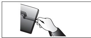
If the steam plate is fitted with a metal swivel joint, tighten hose nut to thread using two spanners. The plate can remain permanently attached to the hose thererafter.
