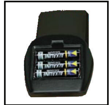
Fig. #57 Remote Control Transmitter battery bay
