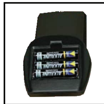
Fig. #50 Remote Control Transmitter battery bay
