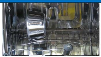
2. Lower horizontal rack and position pot over jet - note angle. Maximum 1 pot per load.
