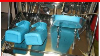
2. Position bedpans with contents on hooks as illustrated. Slide urinals over jets so clip catches. Close door & contents will empty automatically.
