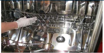
1. Push horizontal rack up to dump commode contents. Bedpan rack must be flat against the door.
