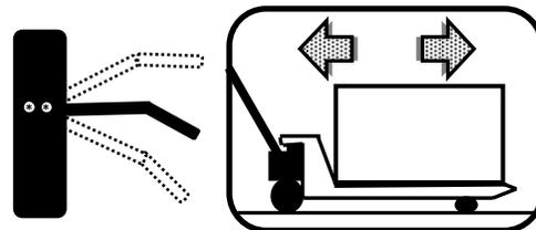
**For free movement**, put Finger Tip Control in the middle, neutral position.
