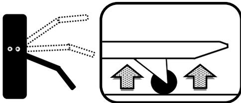
**To raise load**, push down on Finger Tip Control. Pump handle to raise load up from floor.
