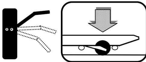
**To lower load**, pull up on Finger Tip Control.
