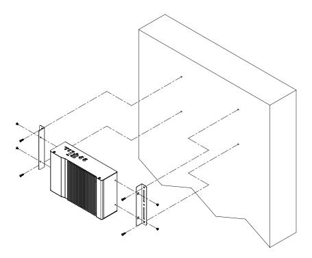
Using attached mounting rail, you can install CSB200 on wood, drywall surface over studs, or a solid concrete or metal plane. Ensure the installer uses at least four M4 length 8mm screws to secure the system on wall. *Six M4 length 8mm screws are recommended to secure the system on wall.*
