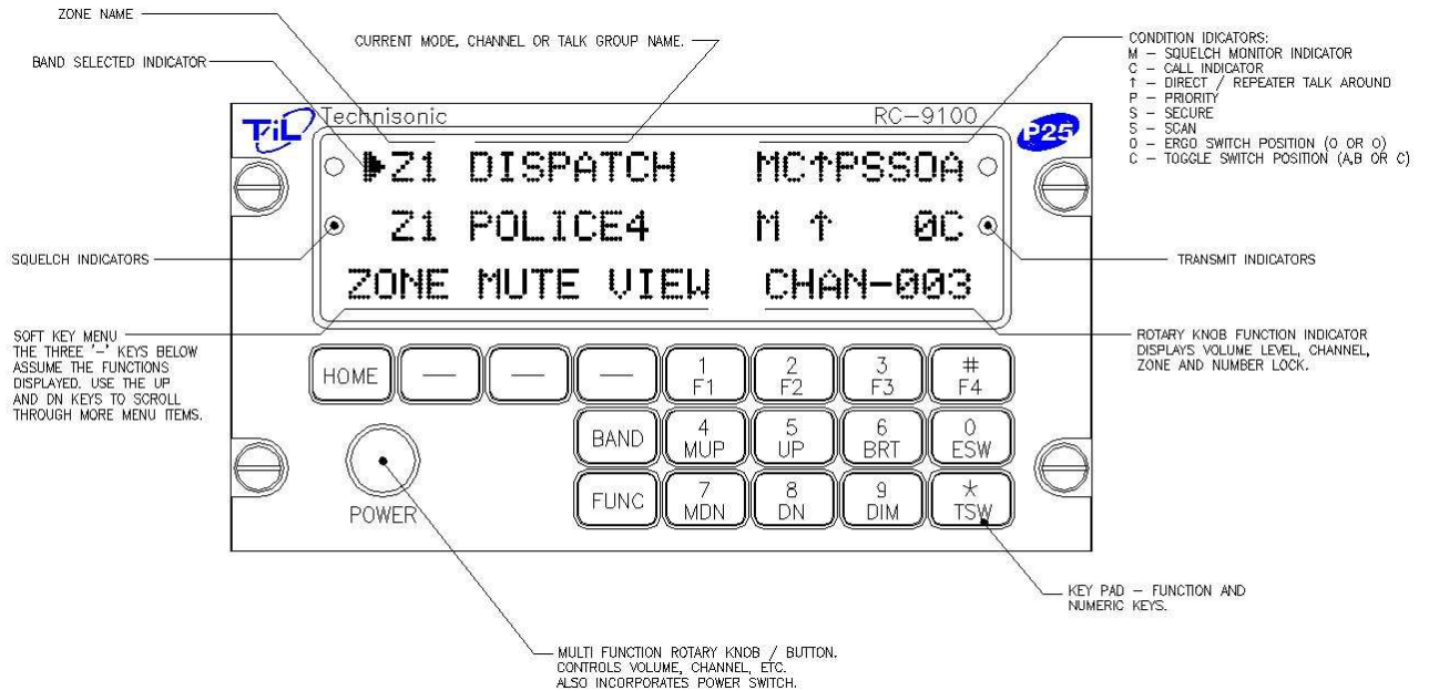
FIGURE 2.1 Front Panel Controls – RC-9100 Remote Control
