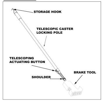
Thread brake tool onto the telescopic pole, hand tight.
