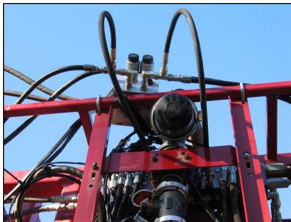
Figure 22: Hydraulic Plumbing Example
