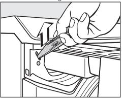
■ Insert a screw driver into the slot of the emergency opener and pull upwards. The door will now open.
