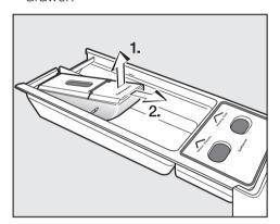
If you do not use bleach, please remove the insert from the main wash compartment. Add detergent to the desired compartments.
