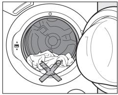
■ Close the drum door. To prevent damage, make sure that there is no clothing caught between the drum door and the seal.
