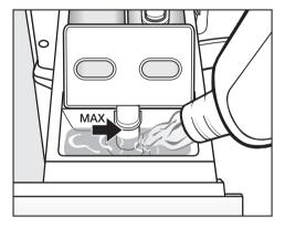
Add the fabric softener or mild liquid starch to the "Softener" compartment.
