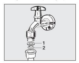
plastic filter, **2**, and pull it out of the hose connector.
