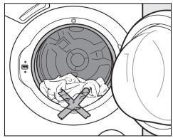
■ Close the drum door. To prevent damage, make sure that there is no clothing caught between the drum door and the seal.
