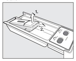
If you do not use bleach, please remove the insert from the main wash compartment. Add detergent to the desired compartments.
