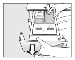
■ Pull the detergent drawer out until it stops, press down the release catch, and remove the drawer from the washer.
