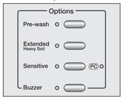
Select the desired Option with the respective button. Once an Option is selected, the indicator lights.
