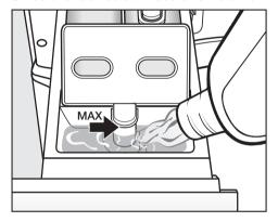
Add the fabric softener or mild liquid starch to the "Softener" compartment.
