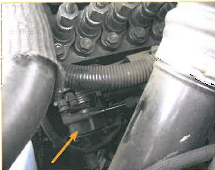
Figure 4: Check for low closed throttle TPS signal voltage on 1997 and earlier diesel applications. TPS is on the injector pump.
