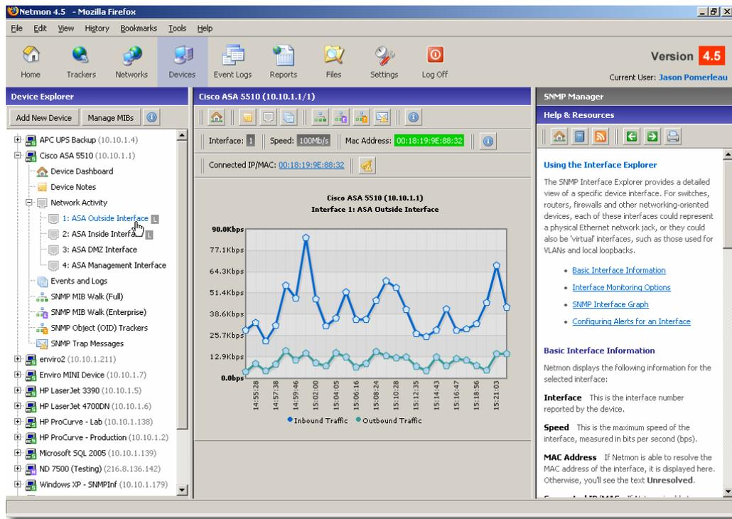
Figure 7 – SNMP Interface Explorer
