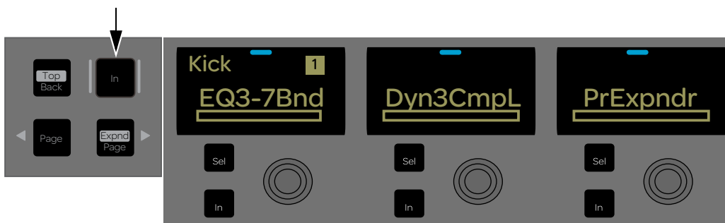
Channel Control Navigation In switch
