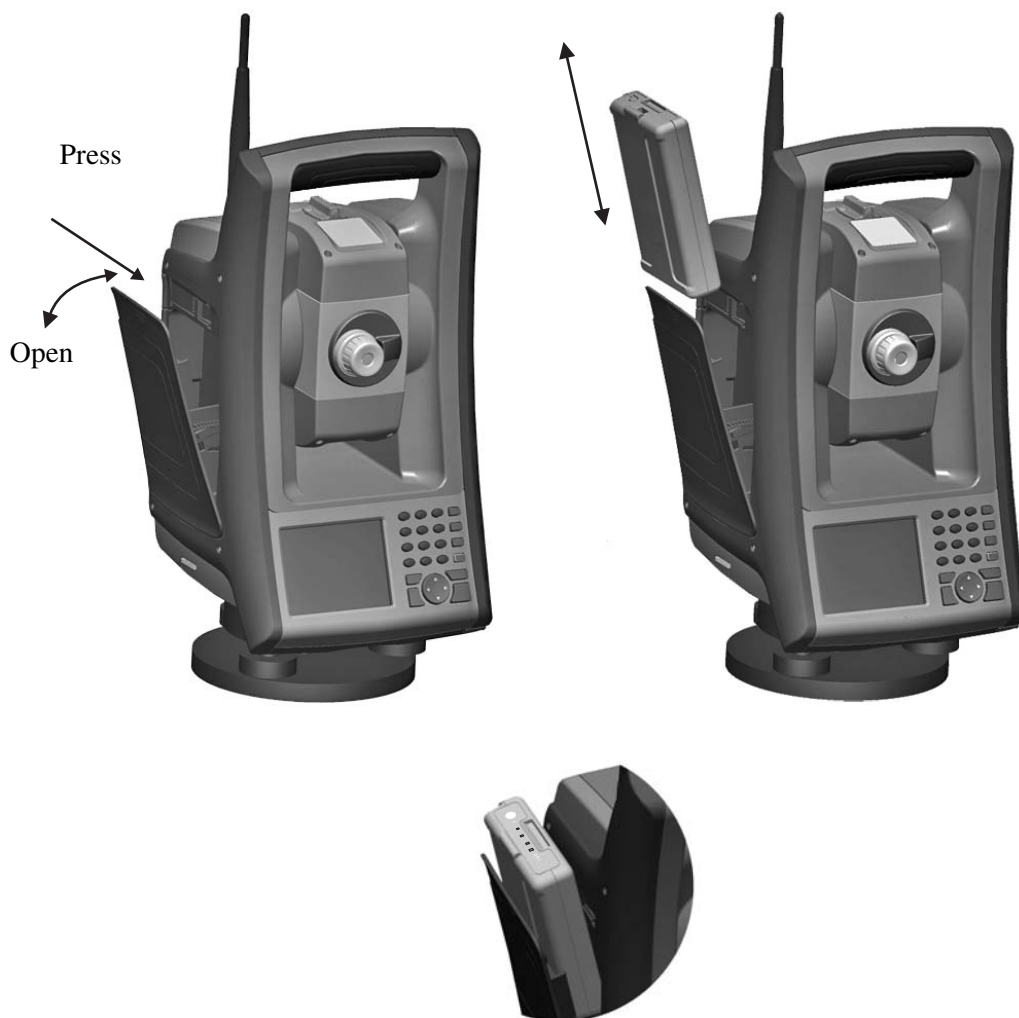
Fig. 3-3 Removing and replacing the internal battery
