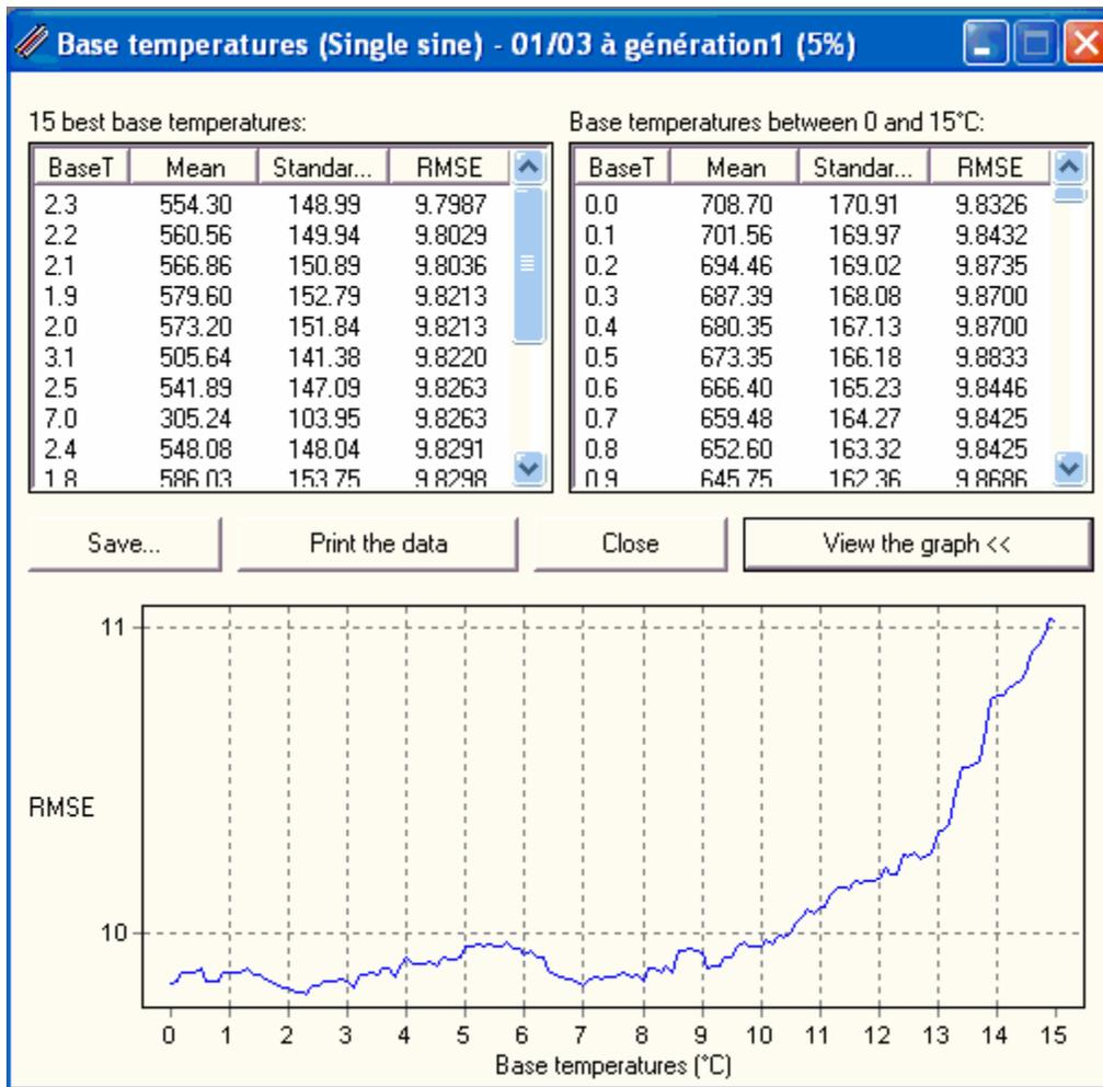
**Figure 10.** Result from estimating base temperatures using RMSE as statistical criteria.
