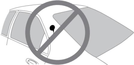
A line drawing of the exterior of a car, showing the front, back, and side pillars. A small black dot representing an antenna is placed on the side pillar. A large, thick grey circle with a diagonal slash through it is overlaid on the image, indicating that this installation is prohibited. |
