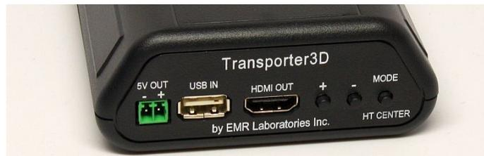
**Transporter3D to Rift Connections: HDMI OUT, USB IN, 5V OUT**
