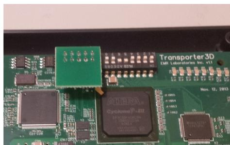
**Identity Module Correct Orientation**
