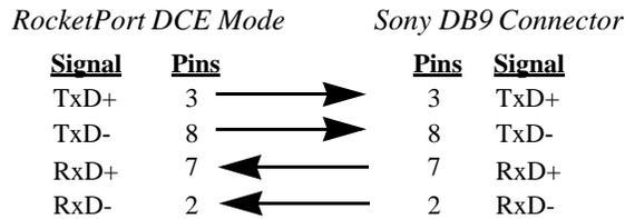
**Null-Modem Cables (DTE)**
