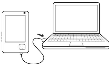
Your eReader will start charging (as long as your computer is running). It can take up to three hours to charge. The status light turns blue when your eReader is fully charged.
