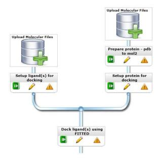
When setting this action in Job manager, a few boxes have to be filled. The number of proteins to be used in the flexible mode is defined in the first box. The protein file name is guessed by the interface as Setup protein for docking should be used in a preceding box.
