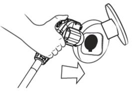
**Step 5**: When the vehicle is charged, remove the connector from the vehicle.
