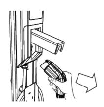
**Step 4**: Plug the connector into the vehicle and charge for the requested period, maximum 3 hours.
