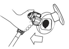
**Step 6**: Roll the cable up on its support, put the connector back into the station and close the door.
