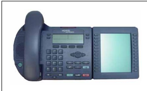
Each of the physical keys on the KEM can have a user-defined label (with a maximum of 10 characters) associated with it. Labels for KEM keys are created using the controls on the IP Phone. KEM keys are numbered sequentially, beginning with the first number after the last defined key on the IP phone. See the IP Phone User Guide for the procedure to create a label for a KEM key.
