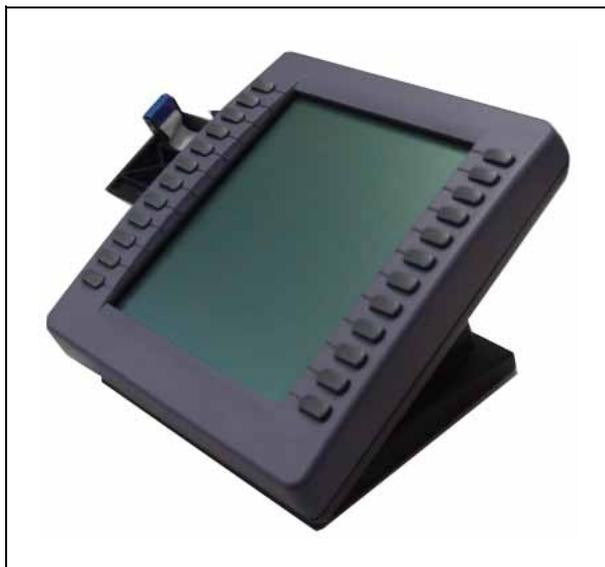
Each KEM has a desk-mount bracket and structural base plate to connect the KEM to a Nortel IP Phone 2002, IP Phone 2004, or to another KEM. You can connect a maximum of two KEMs to the IP Phone 2002 and the IP Phone 2004.
